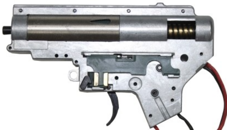
The left side of a standard version 2 gearbox; Note the black selector plate above the trigger. The cutoff lever is on the inside of the gearbox.
